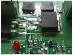
Next, unsolder the large tab on the MOSFET. Due to the large size of the pad, a longer heating time will be required. It may be beneficial to use a larger soldering iron tip for this part.
