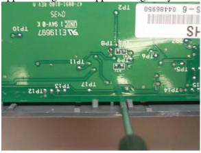
After the circuit board is free from all the tabs, gently remove it from the controller casing being careful not to bend or break off the green wiring terminals.
