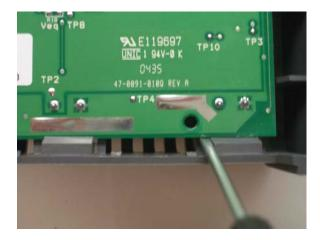
After the edge of the circuit board has been free of all three large tabs, switch to the opposite edge. The opposite edge only has two small tabs in the center.
