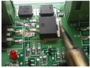
After the MOSFET has been completely removed, remove any excess solder that may remain.
