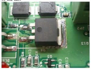
After the circuit board has cooled, carefully place it back in the controller casing and snap it into the plastic retainer tabs. Make sure it is securely seated before putting the back cover on. Reconnect controller and verify its proper operation.
